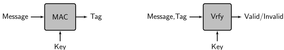
Figure 3.1: The tagging and verification algorithms.
